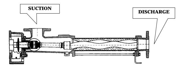
Pipe works have to be same size of delivery-discharge pump's ports.
